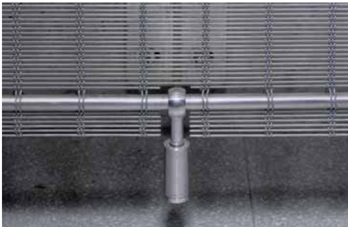
Intermediate fixing: Round bar with integral pendular fixing plates attached to triangular bracket (Type of weave: MULTI-BARRETTE)
